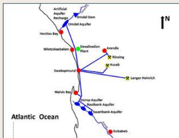
Central Namib Water Supply Scheme
