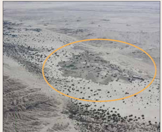
Unregulated sand mining in the Swakop River resulting in a large pit which interferes with the flow of the river when it floods
